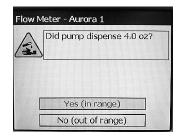
If you select No, it will allow you to enter the measured volume collected. This will set a new calibration factor into the system. It will ask you to perform a post-flush.
