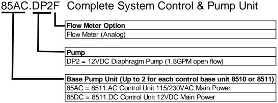
This model number includes both the control unit and a pump unit in a single shipping package. A second pump unit can be added by ordering a 8512 pump unit shipped in a second package.
