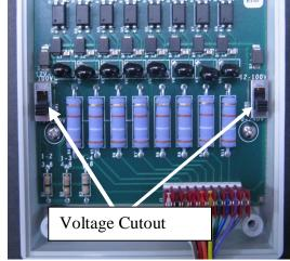
Note: When combining 2 or more trigger signal inputs from one supply signal from the laundry machine, it is recommended to have the voltage cutout switches set to 12V-100V settings. The system will accept 12-250VAC trigger signals.
